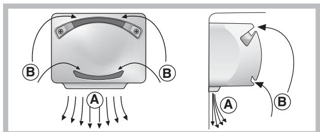
Pure Wind Plus maximises air circulation, improving the efficiency of the evaporator and helping to achieve the optimal temperature inside the refrigerator as quickly as possible each time it has been opened. The blown air (A) is cooled when it comes into contact with the cold wall, whereas the hotter air (B) is sucked up (see diagram).
