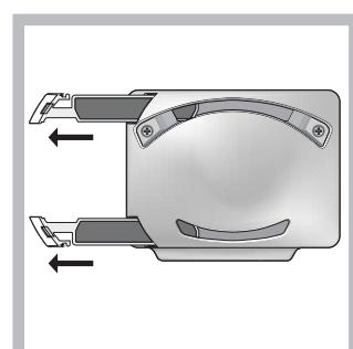
If the filters cannot be removed, or if they are difficult to remove, please contact the Technical Assistance Service.
