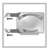
running water, using a neutral detergent to remove any stubborn build-up. Leave the filters to dry before replacing them. If the filters cannot be removed, or if they are difficult to remove, please contact the Technical Assistance Service.
